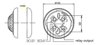
Pin 1&2: relay output Pin 3&4: power input
